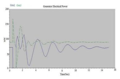
Figure 5: Generator Electrical Power with PSS and Shunt Capacitor
