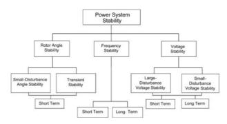
Figure 1: Classification of Power System Stability
