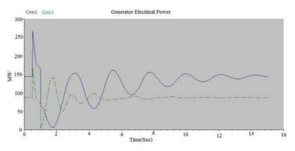
Figure 10: Generator Electrical Power without PSS and Shunt Capacitor
