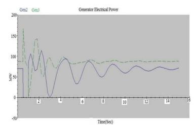
Figure 4: Generator Electrical Power without PSS and Shunt Capacitor
