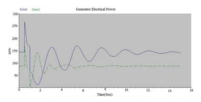
Figure 11: Generator Electrical Power with PSS and Shunt Capacitor
