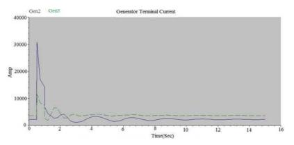
Figure 9: Generator Terminal Current with PSS and Shunt Capacitor
